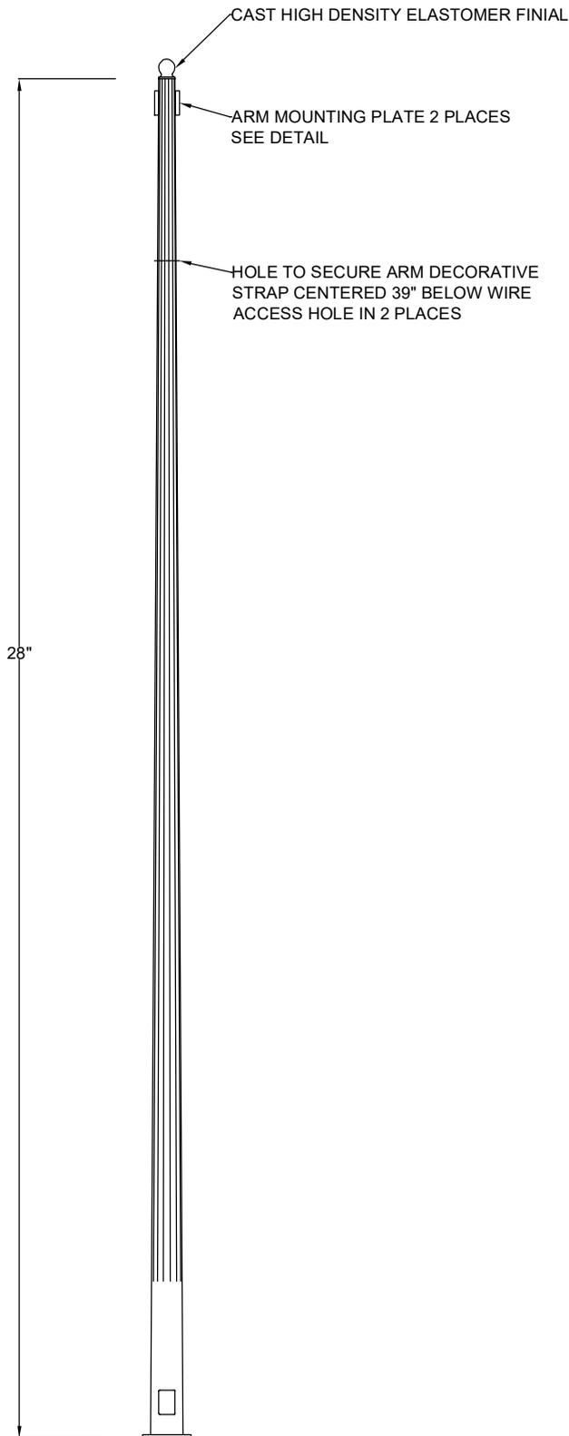
28' TAPERED FLUTED STEEL POLE IS 4" DIA AT TOP AND 8" DIA AT BOTTOM. POLE HAS 16 FLUTES WITH AN 11 GAUGE WALL. MINIMUM 12 EPA @ 80 MPH, 1.3 GF.
